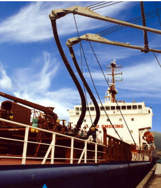
A644 dock hoses for oil transfer
